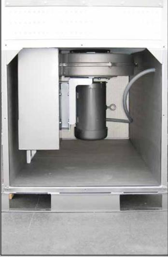
Massive 7.5 HP motor drives large diameter blower that combined with the "stealth technology silencer provides world-class ventilation with a quiet workplace.
