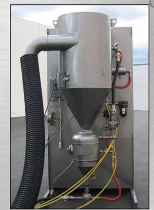
The 7-inch diameter hose and massive cyclone prove this baby sucks! Generous pressure vessel gives tons of blast time even with large nozzles.
