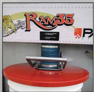
Included locking lift handle and multi-size drum cover means Operators do not deal with dusty drawer disposal. The drum cover is compatible with most drums from greater than 55 gallon downward.
