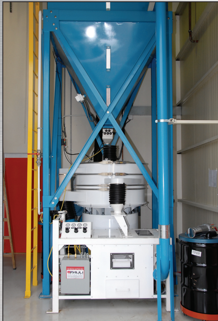
Media Reclaim Sub-System with Pauli Patented Dense Particle Separator.
